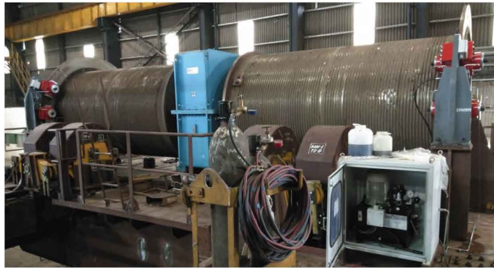
Emergency Disc Brakes (Hydraulic Fail-safe) directly mounted on Rope Drum Flange
