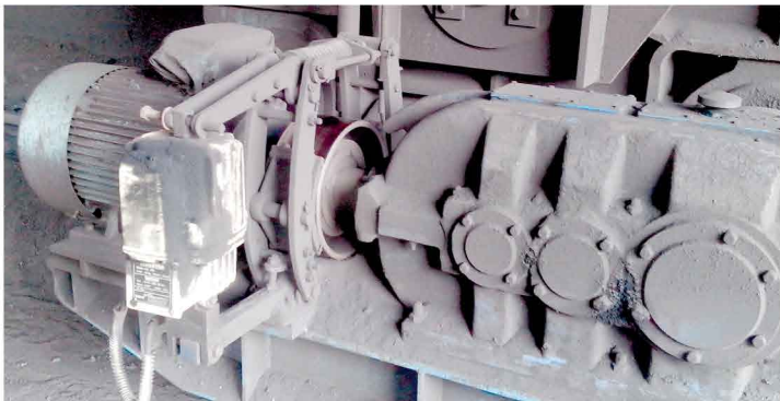
Electro-hydraulic Thruster Drum Brakes mounted on High Speed Side
