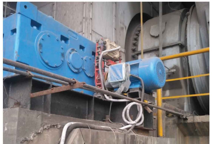
Thruster Drum Brake mounted on Charging and Discharging car in Steel Industry
