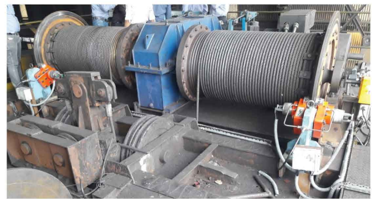
Emergency Disc Brakes (Hydraulic Fail-safe) directly mounted on Rope Drum Flange retrofitted for the existing crane
