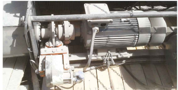
Electro-magnetic Disc Brakes mounted on High Speed Side
