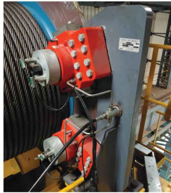
Emergency Disc Brakes (Hydraulic Fail-safe) directly mounted on Rope Drum Flange
