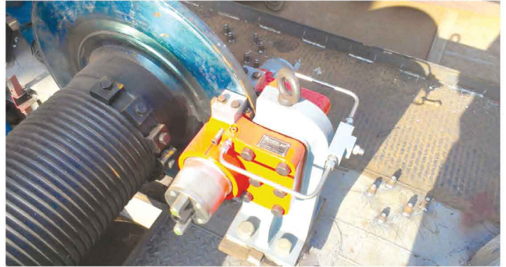
Emergency Disc Brakes (Hydraulic Fail-safe) directly mounted on Rope Drum Flange
